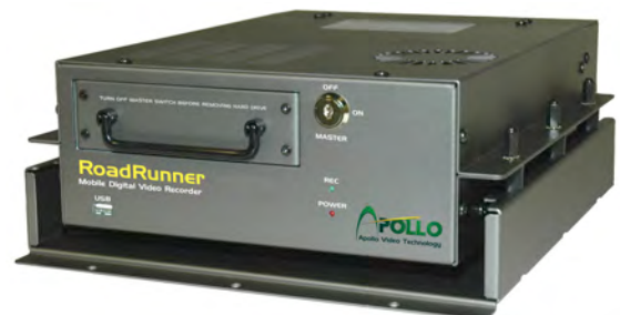
Apollo Video's RoadRunner Mobile Digital Video Recorder
